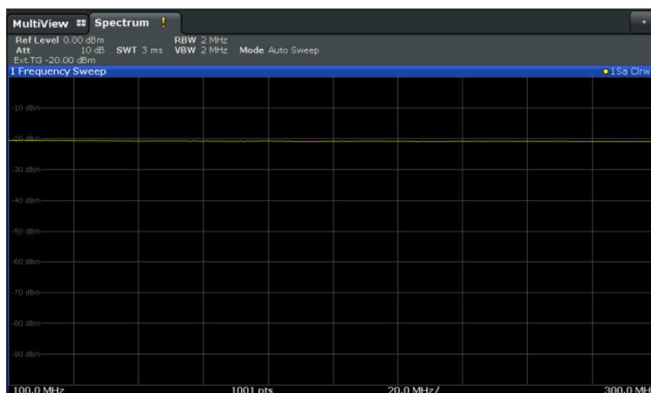
Figure 3-8: Measurement results from generator, analyzer and connecting cables
