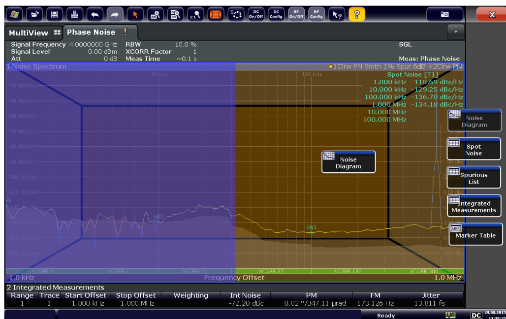
Figure 4-1: Moving a window in SmartGrid mode
